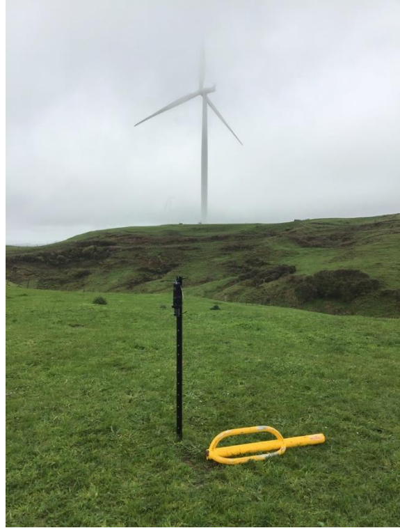
Photograph Appendix C.4: An 'open treatment' acoustic recorder deployed in open pasture a minimum 200 m away from any turbine on Te Uku wind farm.
