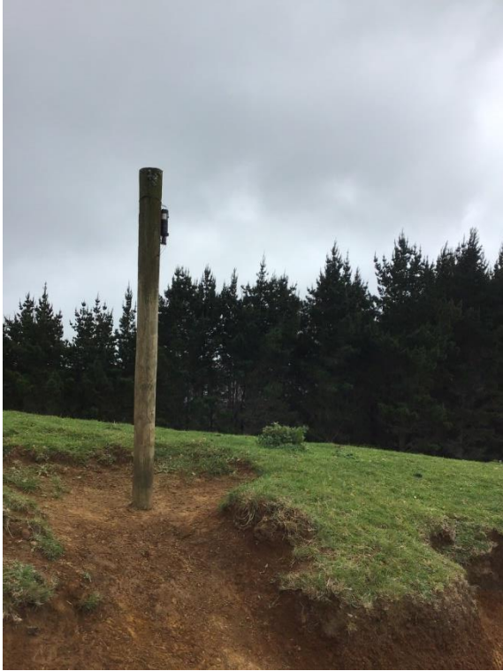
Photograph Appendix C.3: Acoustic recorder deployed on a fencepost adjacent to a turbine at Te Uku wind farm.
