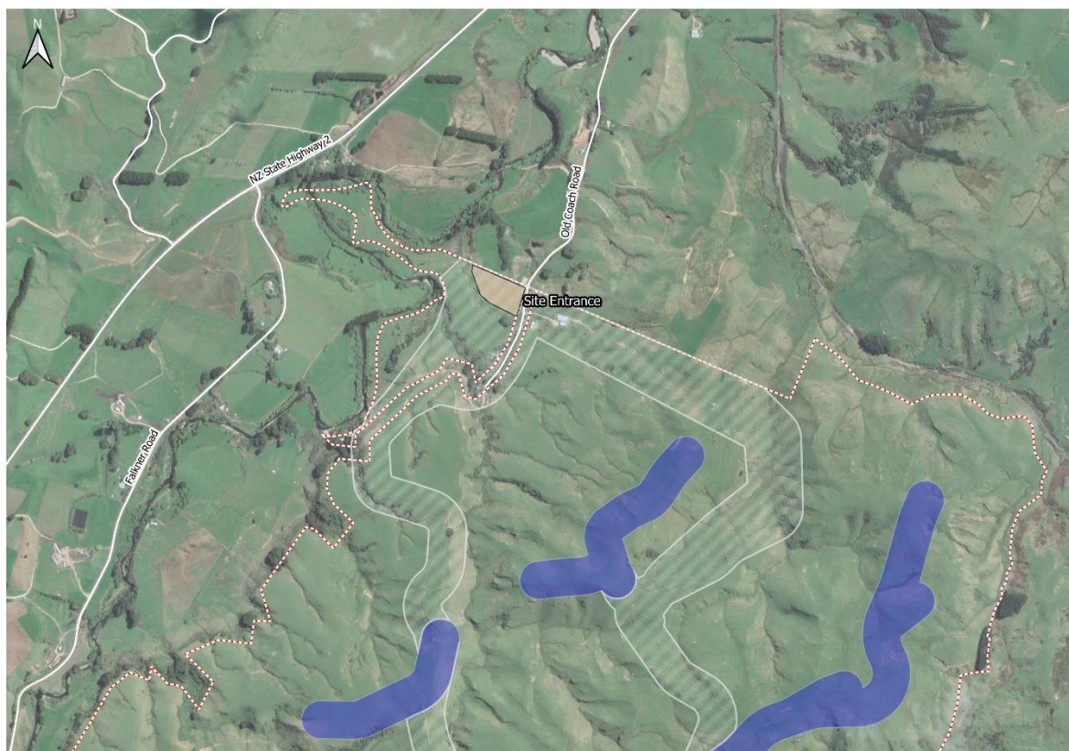
Figure 2.2: Location of the Site Entrance area in the north-western corner of the Site shown in light brown. The Turbine Envelope Zone is in blue, Turbine Exclusion Zone in grey thatching, and the Site boundary is the red and white dashed line (Figure provided by Meridian Energy)
